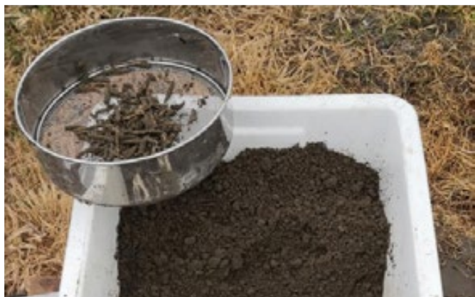
Roots were sifted from the soil samples using a 5mm sieve, and sent to laboratory for washing and analysis.
